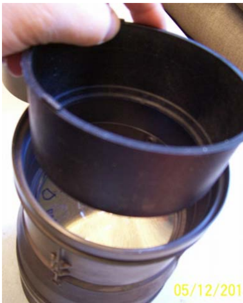
Step 7: lower the plastic spacer in. Lens F will sit on this.
